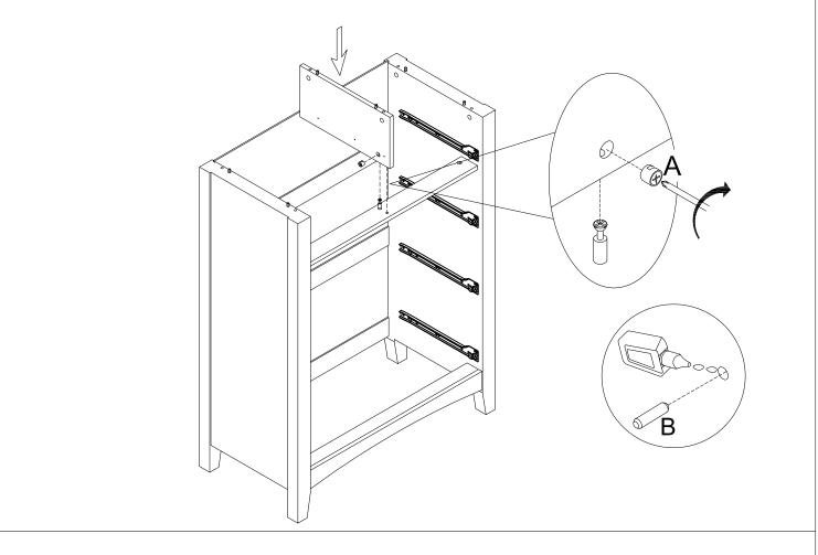
Step 10: Attach the Top Panel(C1).Use a Phillips Head Screwdriver to turn the Cam Lock (A) to lock onto the head of Cam Pin(A).
