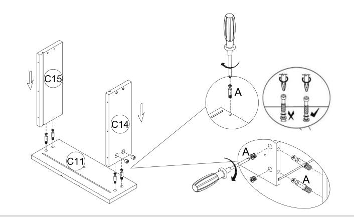
Step 14: Assemble Drawer Left side Panel(C14)and Drawer Right side Panel(C15) to the Drawer Front Panel(C12).Use a Phillips Head Screwdriver to turn the Cam Lock (A) to lock onto the head of Cam Pin(A).
